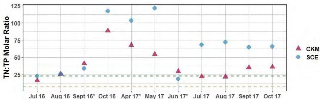
Figure 3-27: Average TN:TP molar ratio of interior sites within each marsh plotted for each sampling event in chronological order. * = sampling followed precipitation event. Above the dark green dashed line (ratio of 22.6; Guildford & Hecky, 2000), P is likely to be limiting. Below the light green dashed line (ratio of 7; Abell, Özkundakci, & Hamilton, 2010), N is likely to be limiting.
