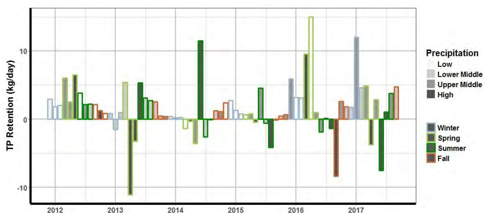
Figure 2-19: TP retention equals monthly average TP load at Spaulding Rd (SCE inlet) minus monthly average TP load at CTH A (SCE outlet). Positive retention signifies SCE stored TP. For negative quantities, it exported additional TP than what flowed in. Gradation indicates precipitation category. Average monthly precipitation over the period was divided into four categories (low, lower middle, upper middle, and high) by quartiles.
