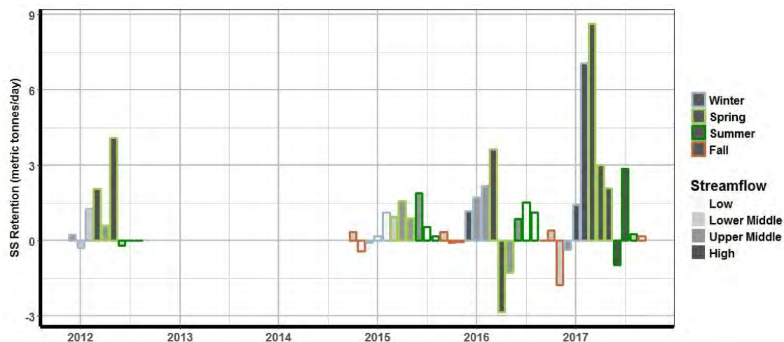
Figure 2-29: SS retention equals monthly average SS load Spaulding RD (SCE inlet) minus monthly average SS load at CTH A (SCE outlet). Positive retention signifies SCE stored SS. For negative quantities, it exported additional SS than what flowed in. Gradation shows relative monthly average streamflow at Spaulding Rd. Average monthly streamflow for period was divided into four categories (low, lower middle, upper middle, and high) by quartiles.
