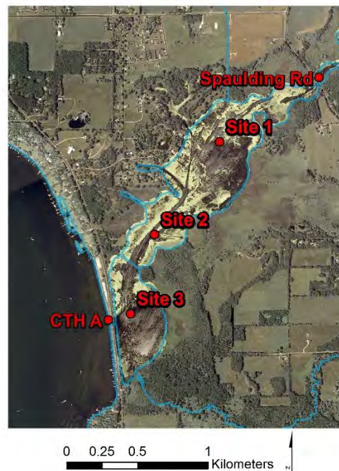
Figure 2-6: USGS monitoring sites are located at Spaulding Rd (inlet) and CTH A (outlet) to monitor flow through Silver Creek Estuary. Water quality samples were collected at those two monitoring sites and at Sites 1, 2, and 3.
